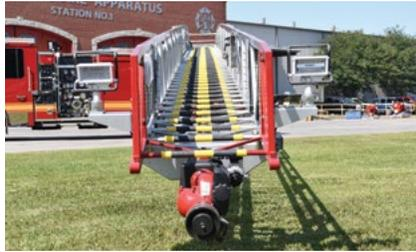
High handrails make it easier and safer to climb the ladder
