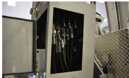
Manual overrides are conveniently located inside the turntable control console
