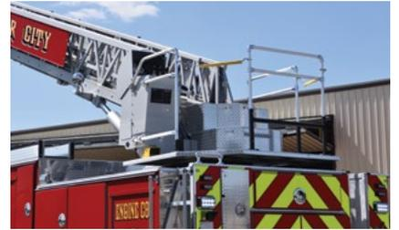
Intermediate steps allows easy movement from turntable to the ladder
