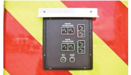
Easy setup with waterproof illuminated outrigger controls
