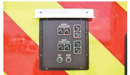
Easy setup with waterproof illuminated outrigger controls
