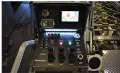
Ladder controls are electric over hydraulic and operated through a deadman switch
