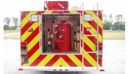
Dry chemical station
