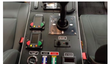
Custom console with pump controls
