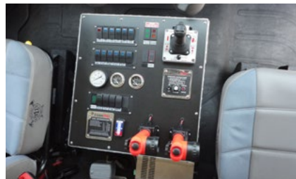
Custom console with pump controls
