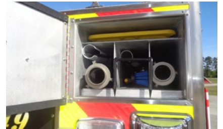
Rear suction and equipment storage
