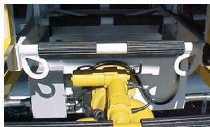
Standard pair of load lifting eyes at the ladder tip are rated at 500lbs as a pair for added rescue capability
