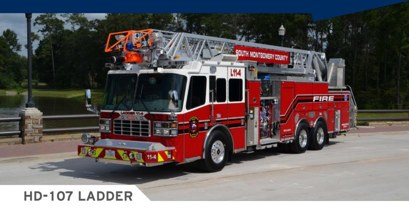
You want Heavy Duty? Then get Heavy Duty! Nothing says that like the Ferrara HD-107. Built with an impressive 750 pound tip load while flowing 1500 gpm in any ladder configuration, the HD-107 can be designed as a traditional truck or a quint with up to a 650 gallon tank.
